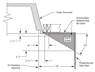
Figure 8 - Side Clearances for Combustible Materials
